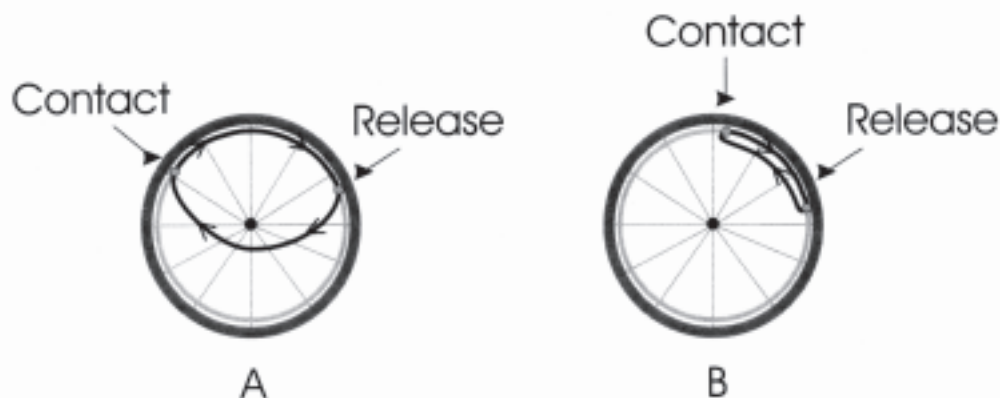
FIGURE 3: THE RECOMMENDED PROPULSION PATTERN IS SHOWN IN "A." AN EXAMPLE OF A POOR PROPULSION PATTERN IS SHOWN IN "B" (ARC PATTERN). THE THICK BLACK LINE ON THE WHEEL IS THE PATH FOLLOWED BY THE HAND.
